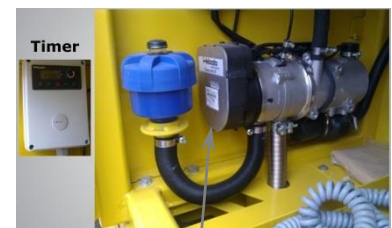
HEATING SYSTEM FOR ENGINE
